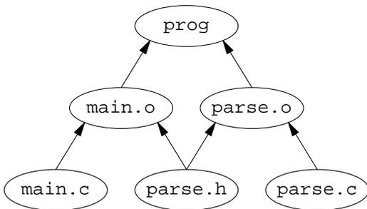
This is an *acyclic* graph because of the arrows which express the ordering of the relationship between the files. If there was a circular dependency according to the arrows, it would be an error.
